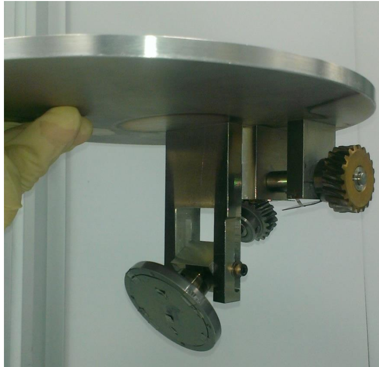
Figure 3.4 Custom made substrate holder with controllable tilting angle.
