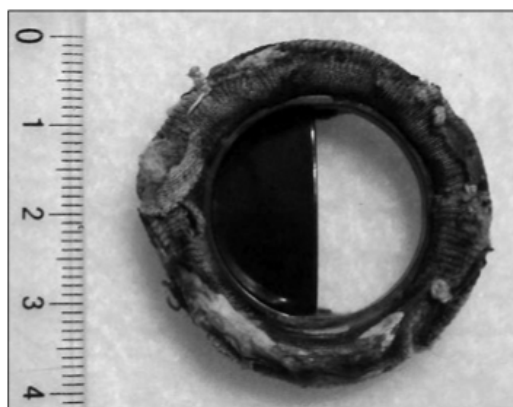
Figure 1-14: Damaged 31mm Edwards-Duromedics mechanical valve showing the remaining leaflet (Lee et al. , 2011)
