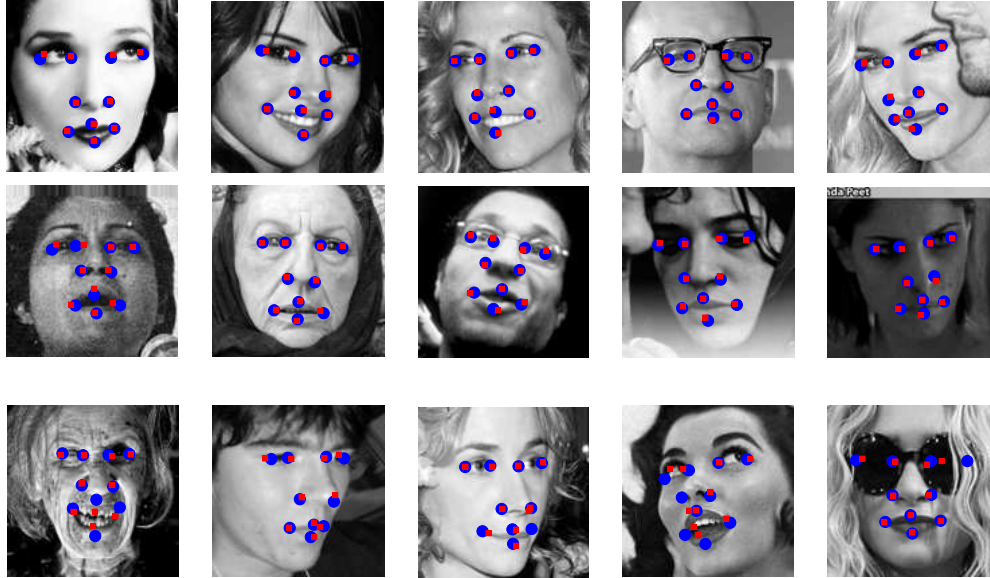
Figure 6.6: Detection examples of the LPFW dataset. The first two rows show the successful detections under challenging circumstances of expression, occlusion, pose, lighting and poor quality. The third row shows some failed cases. The red and blue marks respectively show the detected landmark and the ground truth (best viewed in color).
