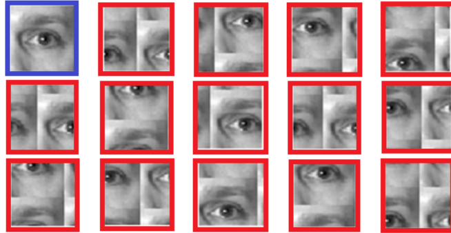
Figure 2.2: The shifted versions of the cropped right eye patch which are explicitly produced over the circular property of correlation operation. The first example (top left) with a blue border shows the training patch with zero circular shift (no shift) and is used as a target example. The other examples with a red border are shifted versions of the target patch and are used as non-target examples over the training process. The shifted patches which we refer to as synthetic patches are not representative of real non-target patches stemming from different parts of images. Training correlation filters by these shifted patches may result in strong peaks at non-target patches, decreasing the robustness against translation.
