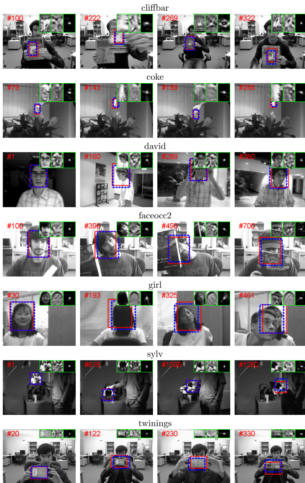
Figure 5.10: Tracking results of our method over testing videos with challenging variations of pose, scale, illumination and partial occlusion. The blue (dashed) and red boxes respectively represent the ground truth and the positions predicted by our method. For each frame, we illustrate the target, trained filter and correlation output.
