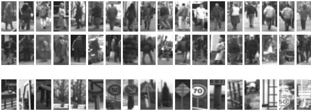
Figure 3.5: Some samples of (top) true detection of pedestrian (true positive), (middle) false detection of non-pedestrian (false negative), and (bottom) false detection of pedestrian (false positive).
