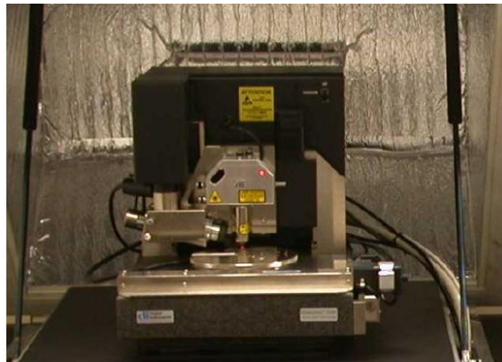
Figure 3-17: The AFM used in this work. The system is shielded from outside noise.
