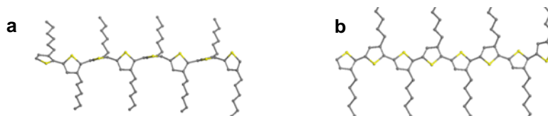
Figure 11. Optimised structures of P3HT molecule of 8 thiophene rings as calculated by a) MRC forcefield and b) our modified forcefield. While our modified forcefield was able to reproduce DFT results with the trans configuration as the most preferred, MRC forcefield relaxed to 90° torsion configuration which was highly unstable according DFT results. Hydrogen atoms are not show for clarity.
