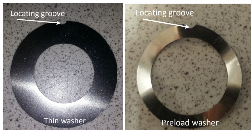
Figure 7.24: Prototype of Thin washer and bearing preload washer
