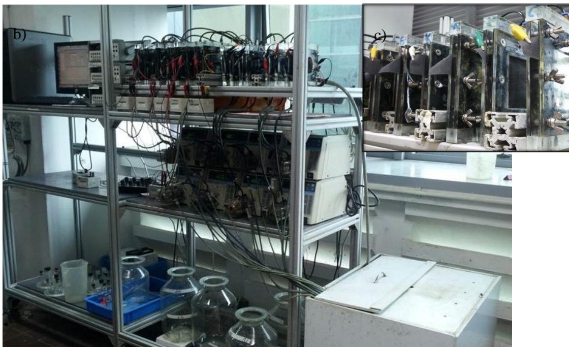
Figure 3.1. a) Schematic diagram of the sensing system using MES (size not to scale) b) A photo of the laboratory-scale MES. c) A photo of the group of MES.
