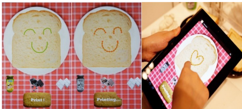
Figure 6.3: (L) Screenshot of pattern tracking and segmentation, before and after “Print” is pressed (R) User use this interface to draw a “Heart”.
