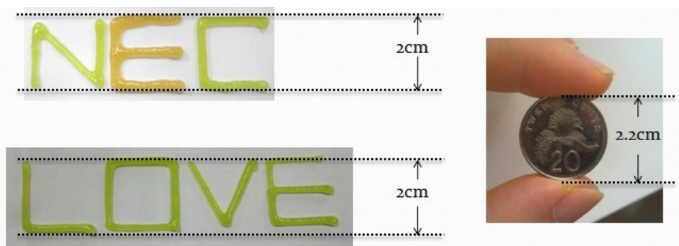
Figure 6.5: (Top) Syringe rotation implemented to print with multiple materials; (Bottom) Print with single material.
