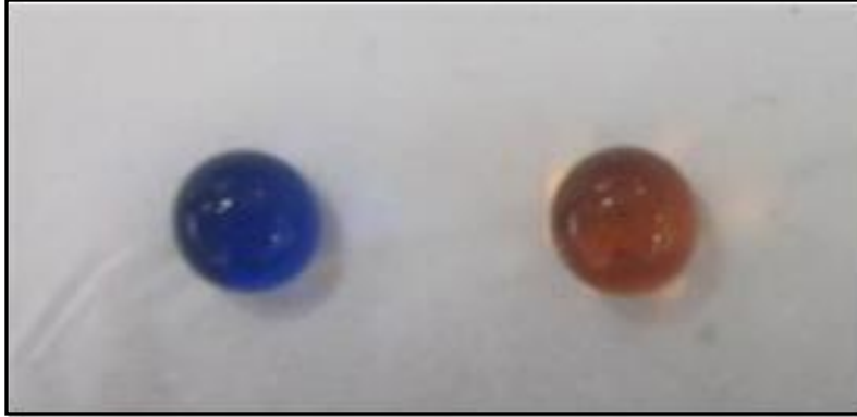
Figure 3.5: Trypan and Alizarin red dye solutions (in water) on FPSi8 fluoroPOSS-PVDF electrospun membrane.
