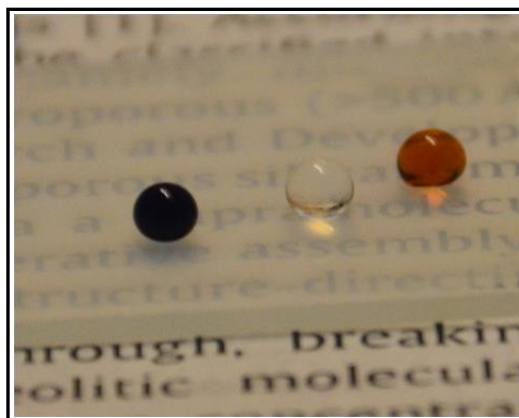
Figure 6.6: Photograph of water (blue - dyed with trypan blue dye), hexadecane (red - dyed with alizarin red dye) and ethylene glycol (colourless) droplets on the superamphiphobic surface.
