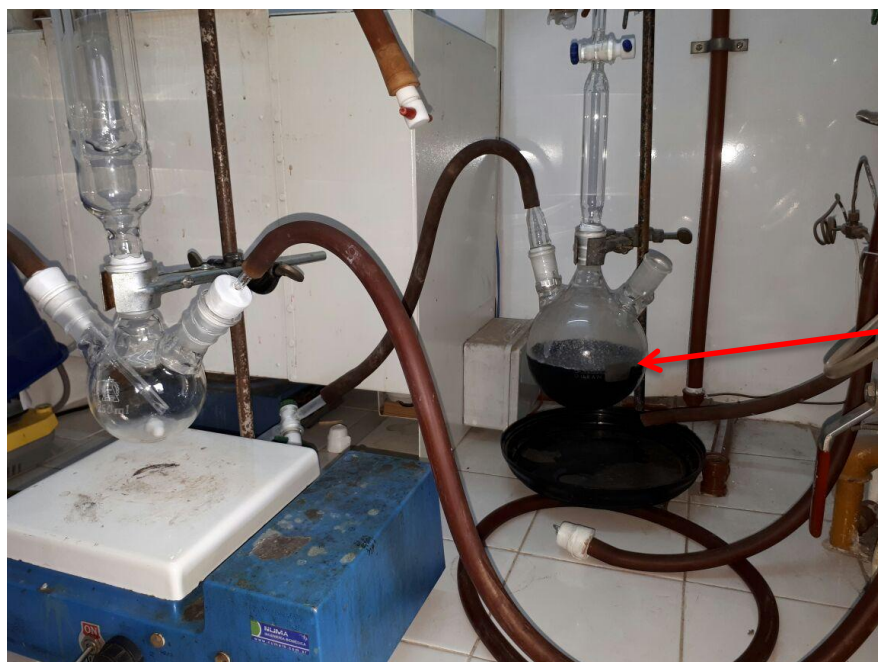
- Picture SI-3 : Experimental device for the \text{NH}_3(l) reactions. Solvent drying process.
