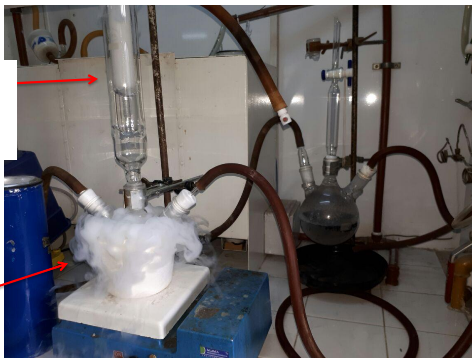
- Picture SI-4 : Experimental device for the \text{NH}_3(l) reactions. Distillation of \text{NH}_3(l) dry.
