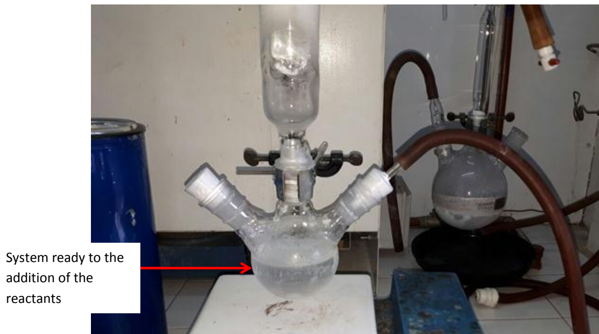
Picture SI-6 : Experimental device for the \text{NH}_3(l) reactions. Dark reaction.
