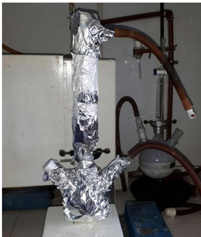
Picture SI-6 : Experimental device for the \text{NH}_3(l) reactions. Dark reaction.
