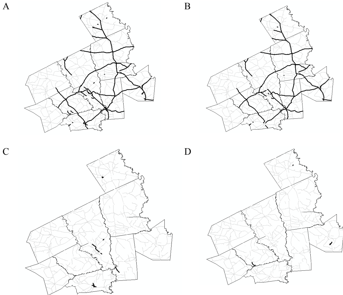
Figure 25. Network roads included in the analysis: (A) total network, (B) state highways, (C) business routes, (D) park and recreational roads
