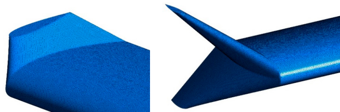
Figure 3. Details of the surface mesh generated in the blade tip devices: (left) asymmetric and (right) symmetric.
