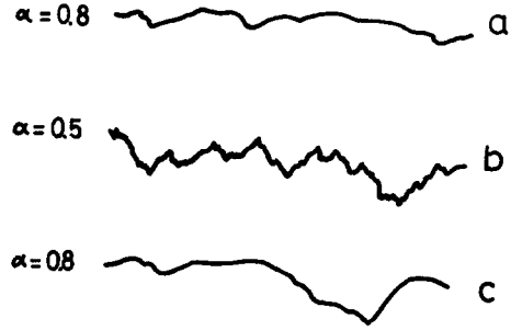
Fig. 7. STM profiles of Au electrodeposits: (a) slow growth rate ( 0.01 \text{ nm s}^{-1} ); (b) fast growth rate ( 100 \text{ nm s}^{-1} ); (c) fast growth rate ( 100 \text{ nm s}^{-1} ) after 7 \times 10^4 \text{ s} aging in 0.5 \text{ M H}_2\text{SO}_4 at 50^\circ\text{C} . Values of \alpha for each profile are also given.
