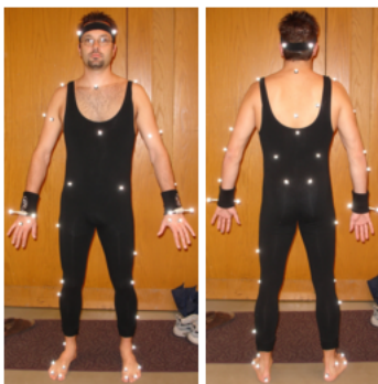
Figure 2: Example of arrangement of sensors on performers body. Taken from MOCAP official website.
