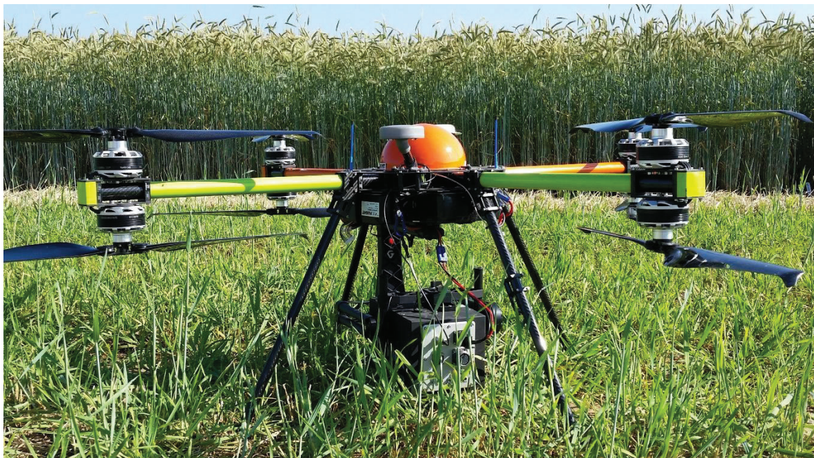
Fig. 2 Hyperspectral sensor-bearing UAV for biomass estimation in large-scale rye field trials.
