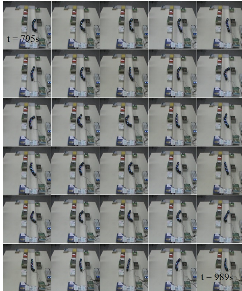
FIGURE 5.41. Robot moving forward in the real straight primenv in a 10 minute test. Frames go from left to right starting in the upper-leftmost one.
