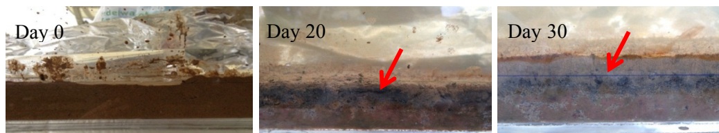
Figure 6.12. Changes in vertical profiles of sediment texture. Distinct black layer of sediments below top layer indication anoxic zone
