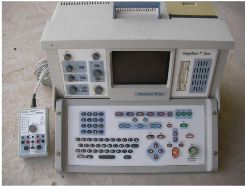
Fig. 3.3. External pulse generator for trigeminal nerve stimulation
