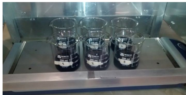
Figure 1. Photocatalysis in aqueous solutions of RB5.
