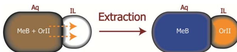
Figure 3.1. Selective and rapid extraction of OrII (orange II) into IL compartment from a mixture with MeB (Methyl Blue) as compound droplet translates along the microchannel.
