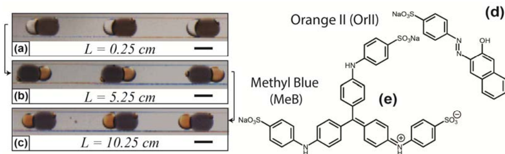
Figure 3.9. (a-c) Stereomicroscopic images of selective liquid-liquid extraction of orange II out of an aqueous binary mixture with methyl blue into the ionic liquid compartment along the microchannel. All scale bars represent 300 \mu\text{m} . d, e) Chemical structures of Orange II (OrII) and Methyl blue (MeB), respectively.
