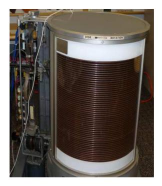
Figure 4.1: First HDD presented by IBM [2]
