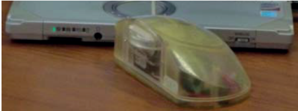
Figure 2.10: Haptic Mouse with Quick and Flexible Tactile Feedback Generated by Double Control Loop
