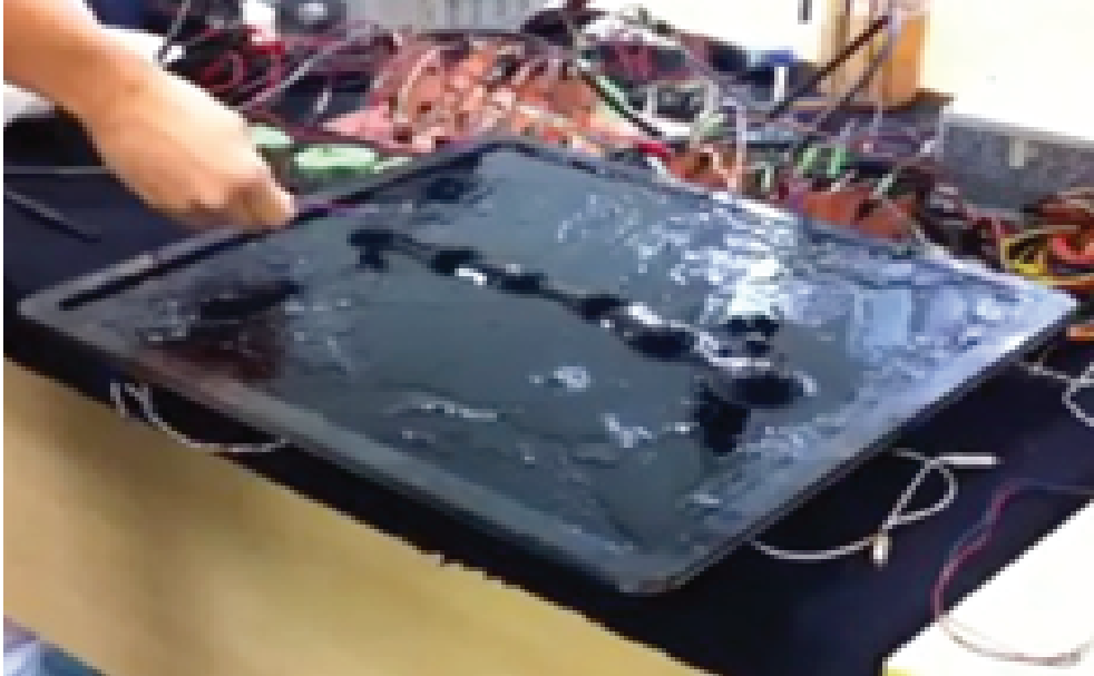
Figure 3.5: Liquid Interfaces system hall effect sensor based input
