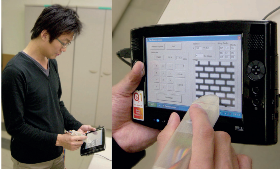
Figure 2.8: Ubi-Pen: A Haptic Interface with Texture and Vibrotactile Display
