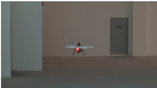
Figure 7.12: Wall-following flight test: go around the corners
