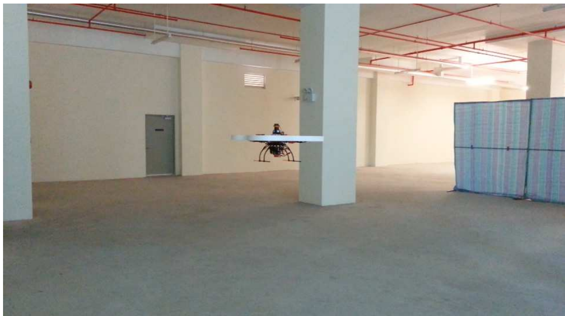
Figure 6.26: Quadrotor position hold via optical flow (Moment 1)
