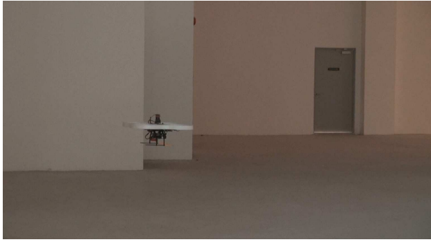
Figure 7.11: Wall-following flight test: encounter a frontal wall
