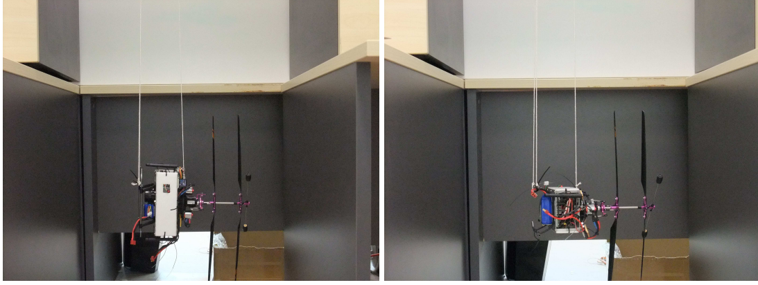
Figure 4.5: The trifilar pendulum method in helicopter x - and y -axis
