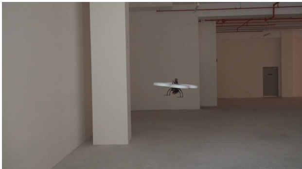
Figure 7.9: Wall-following flight test: avoid a pillar
