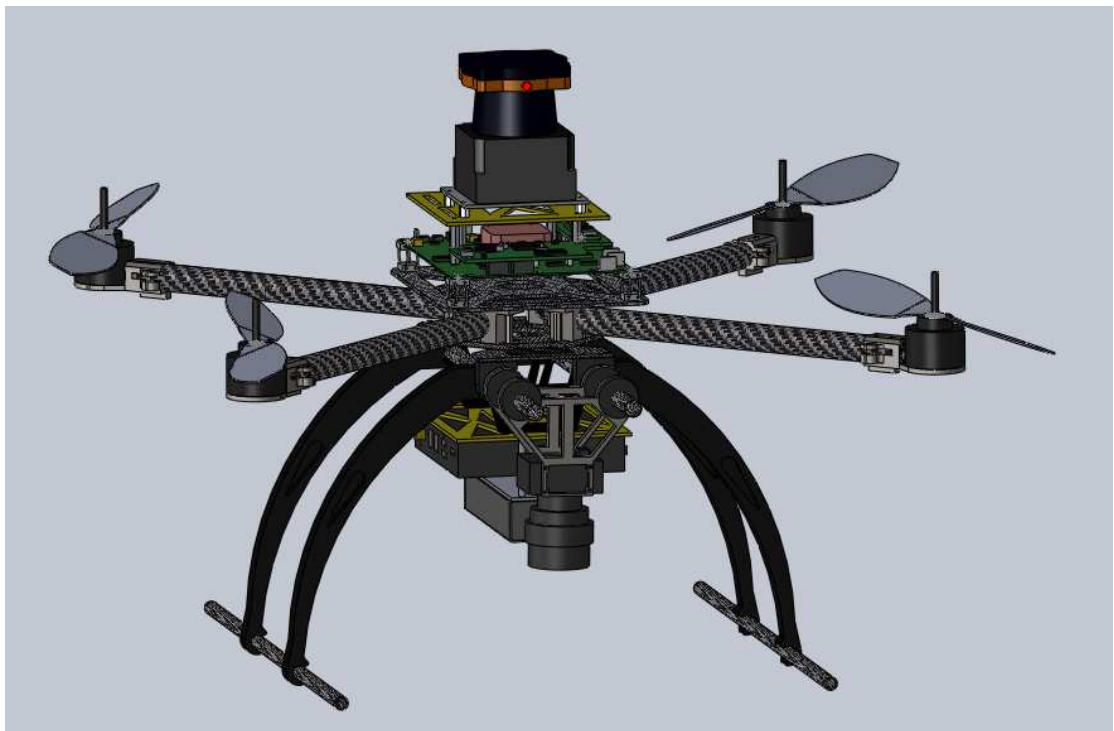
Figure 3.26: SolidWorks design for the whole quadrotor platform
