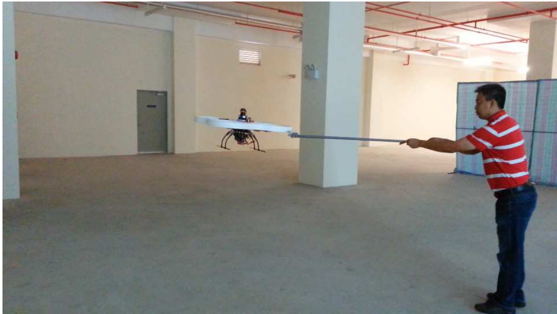
Figure 6.27: Quadrotor position hold via optical flow (Moment 2)
