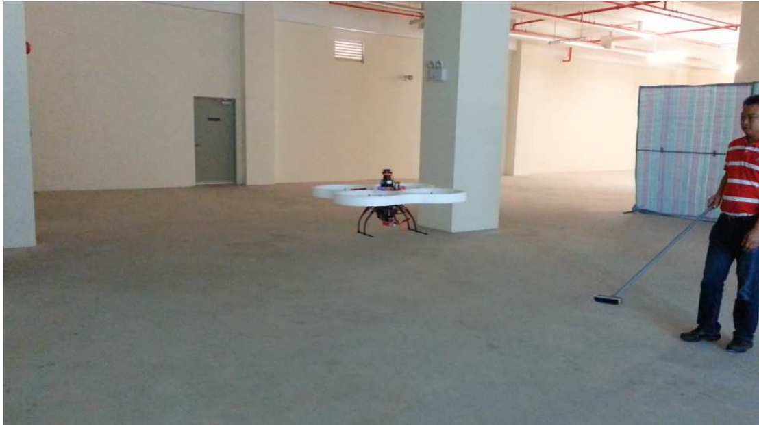
Figure 6.29: Quadrotor position hold via optical flow (Moment 4)
