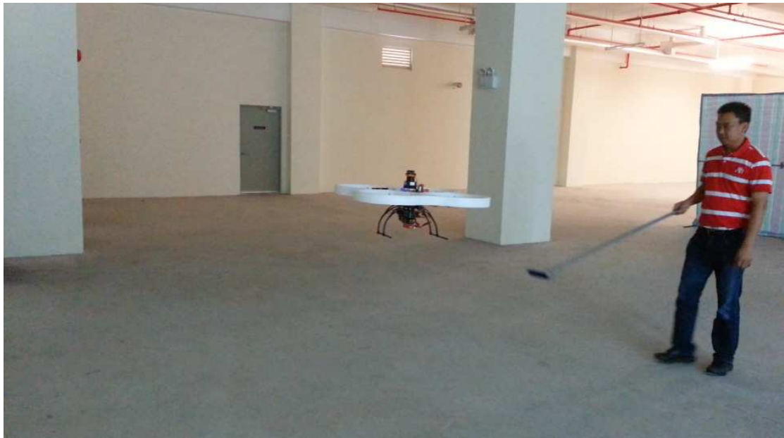
Figure 6.28: Quadrotor position hold via optical flow (Moment 3)
