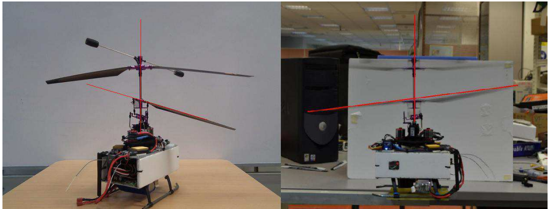
Figure 4.12: Left: Maximum teetering angle of the lower rotor hub; Right: Maximum flapping angle of the lower rotor
