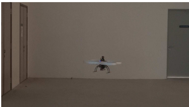
Figure 7.13: Wall-following flight test: encounter the 2nd frontal wall
