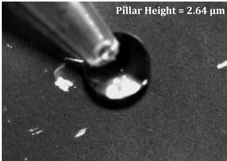
Figure 6.2 Water droplet of 1 \mu\text{l} forms a perfect sphere on the tip of the pipette.
