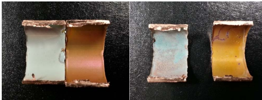
Figure 5.14 Scale formation on a copper pipe segment of System C in the presence of (a) monochloramine (4 mg/L as \text{Cl}_2 ) and (b) free chlorine (2 mg/L as \text{Cl}_2 ).
