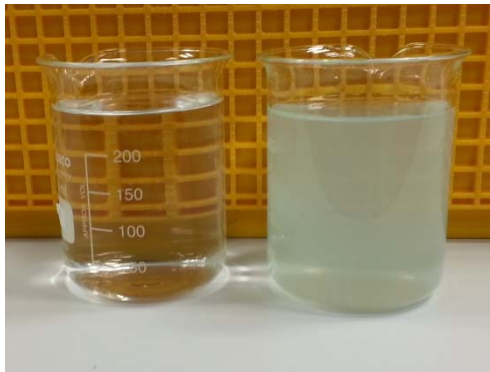
Figure 5.12 Samples collected, before (right) and after filtration (left), from System A after replacement of pipe segment.
