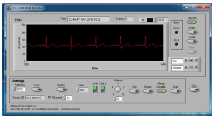
Fig. 3. GUI interface for PC.
