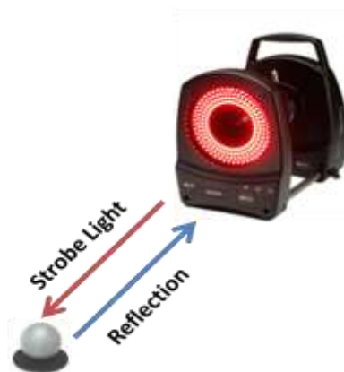
Figure 3.12 Camera obtaining the strobe light reflected by marker
