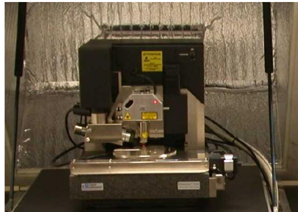
Figure 2-10: Veeco® scanning probe microscopy system. The system is shielded during measurements isolate the measurement system from the outside magnetic noise.
