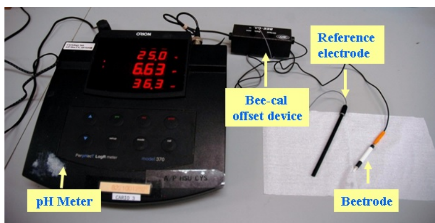
Fig. 2.2. Micro-pH meter set up. The Beetrode and reference electrode were connected to the pH meter via the Bee-cal offset device.
