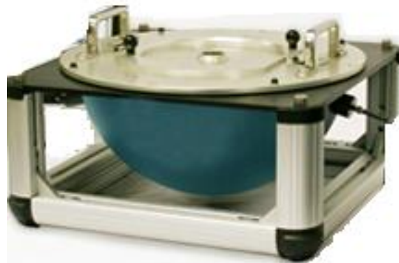
Fig. 7.29. Integrating hemisphere system
