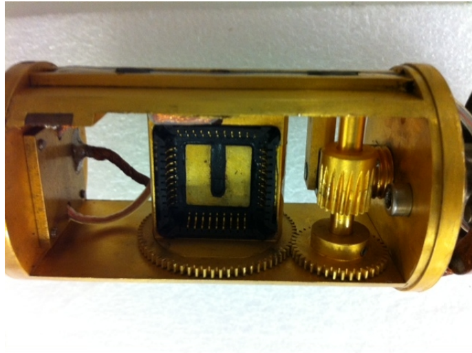
Figure 3.12: The sample holder in the rotating probe. The sample holder can be rotated to align the sample parallel to- or perpendicular to- the direction of the applied magnetic field.
