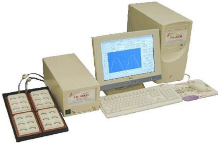
Figure 2.3. Flexcell® FX-4000™ Tension system. UniFlex® plate with confluent human PDL cells were assembled in the standard BioFlex® baseplate with Arcangle® Loading station. The set up was connected to the FX-4000™ Tension system and subjected to a programmed regimen of 12% for 5 s (0.2 Hz) every 90 s.
