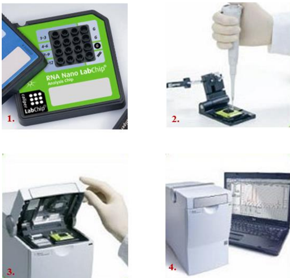
Figure 4.4. Images of summarized steps involved in RNA integrity check process. (1) RNA 6000 Nano LabChip ® ; (2) Sample set up in chip priming station; (3) Chip with samples placed in Bioanalyzer; (4) Bioanalyzer read by a software program installed in the connecting PC.
