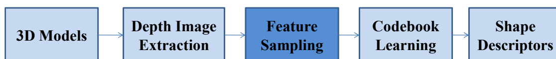
Figure 4.1 Flow chart of sampling strategies of local features for bag-of-words model representation.
