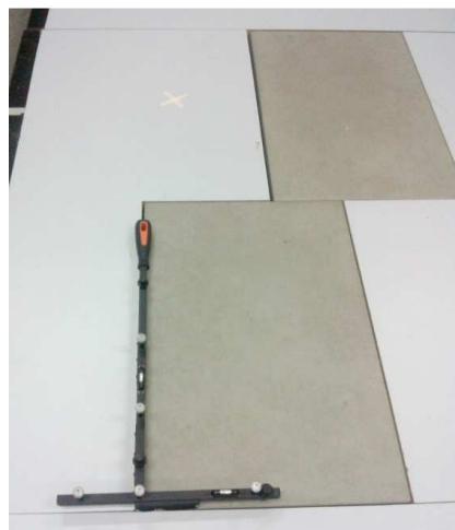
Figure 3.11 5-marker L-frame used to calibrate the cameras and set the Vicon origin
