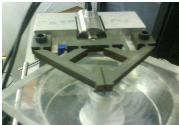
Figure 3-16: “Close-up” of fabricated microgripper and PEA assembly
