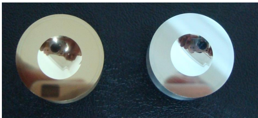
Figure 6-26: Mirror-finish concave profile machined on brass and aluminum workpiece
