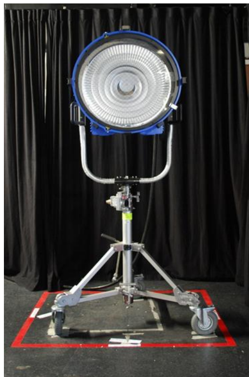
Figure 4:10 – Front view of solar simulator used for SHGC measurements
