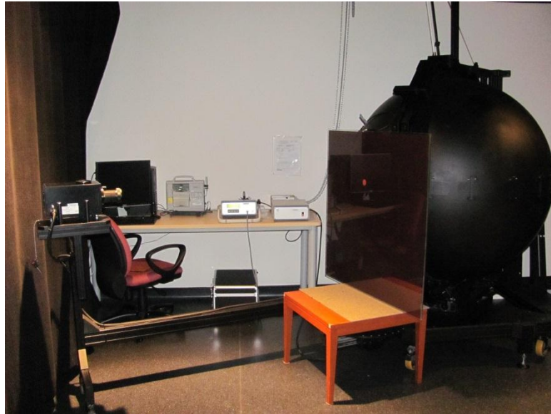
Figure 4:12 – View of semi-transparent BIPV module during VLT measurement using a large integrating sphere
