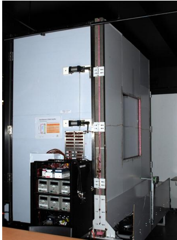
Figure 4:9 – General view of SERIS calorimetric hot box in SHGC measurement mode
