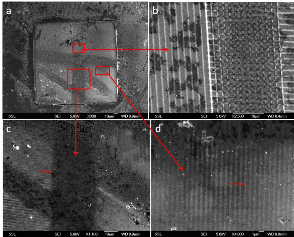
Fig 4. 10 SEMs of the forced current result, surrounding large area: 1 \times 10^{16} protons/cm 2 , 1 MeV protons, square area: 1 \times 10^{15} protons/cm 2 , 500 keV protons, proton beam writing with 0.5 \mu m line width and 1 \mu m and 2 \mu m gaps, (a) overview, (b,c,d) fine views.
