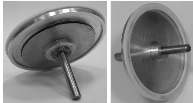
(a) Bonding of rotor and polymer (b) Contact surface on polymer
