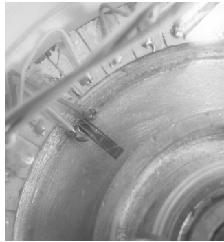
Figure 5.18: Strain gage for axial force measurement
