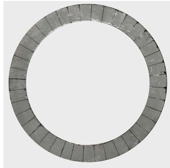
Figure 5.13: Fabricated piezoelectric ring in USM prototype
