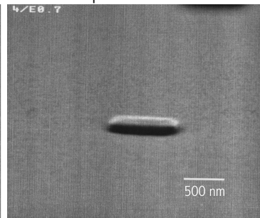
Fig.8c: 0.8 µm wide niobium dot after resist remove
