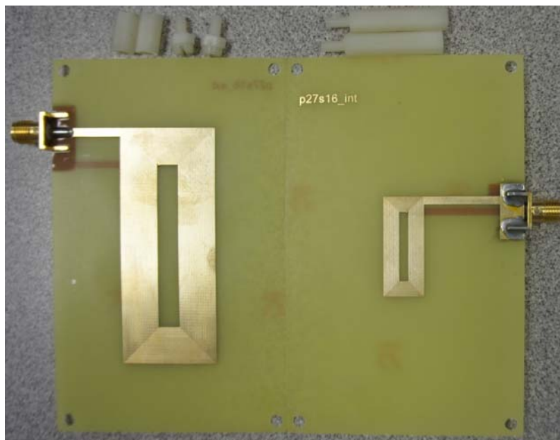
Figure 2-9 Fabricated coupling coils with supporting and connecting materials.
