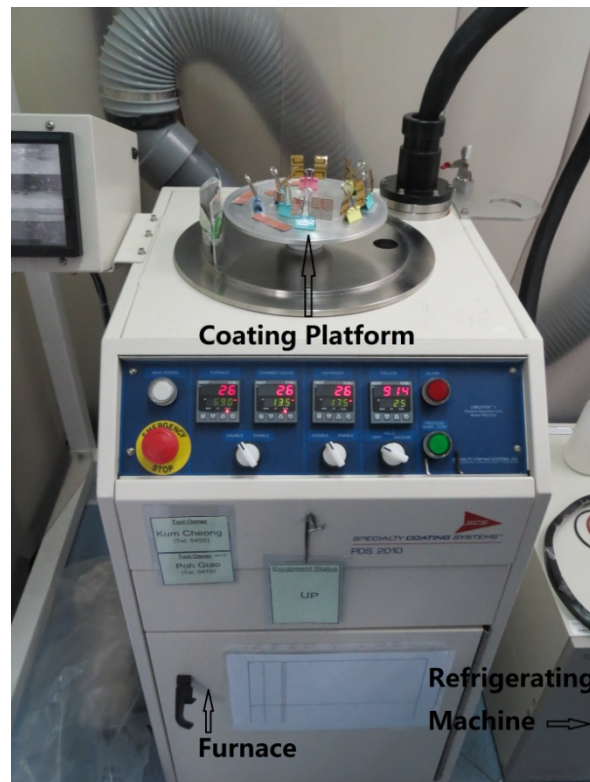
Figure 4-13 Machine used for coating the implantable antennas.
