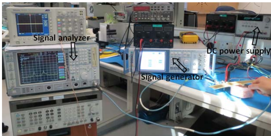
Figure 3-16 System overview of the co-testing platform.
