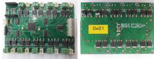
(a) Circuit 1 : 12cmx8cm circuit to drive 9 Peltier modules
