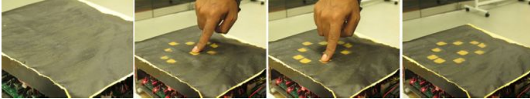
Figure 6.18: Interacting with the Drawing-pad application to draw a heart shape on the textile
