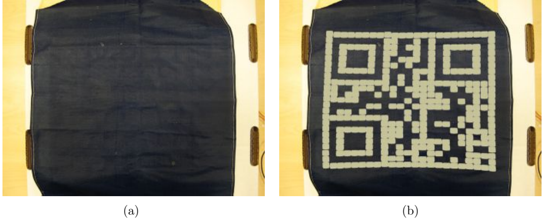
Figure 5.19: Testing the system on fabric materials (a) Without actuation (b) Actuated system
