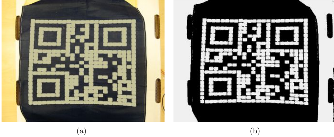
Figure 5.22: Converting the image to complete black and white image (a) Before conversion (b)After conversion
