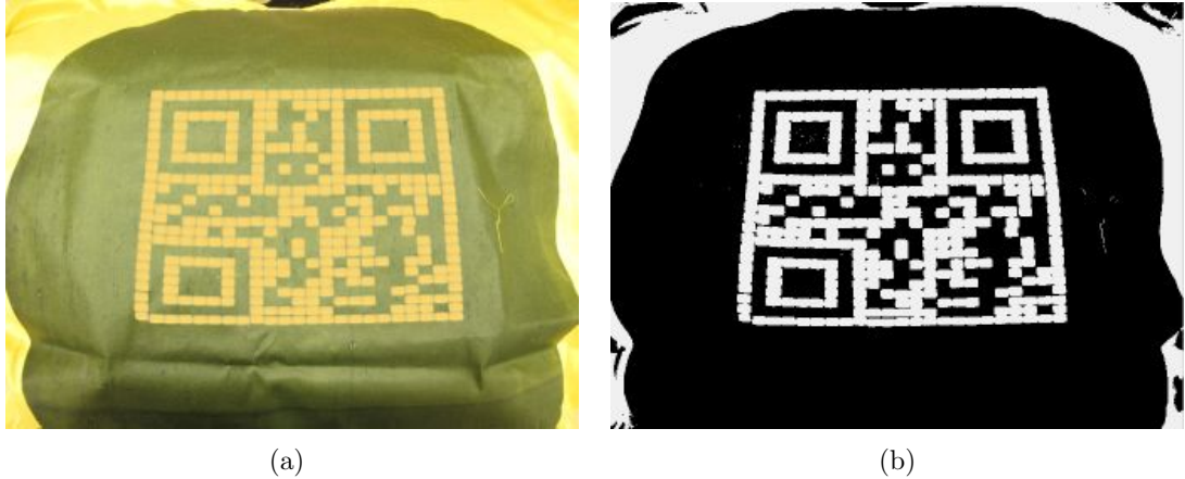
Figure 5.23: Converting a colored image to complete black and white image (a) Without actuation (b) Actuated system
