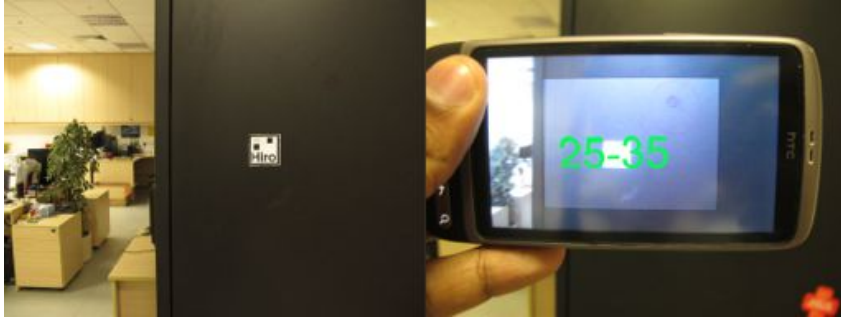
Figure 5.30: Measuring the temperature of a server
