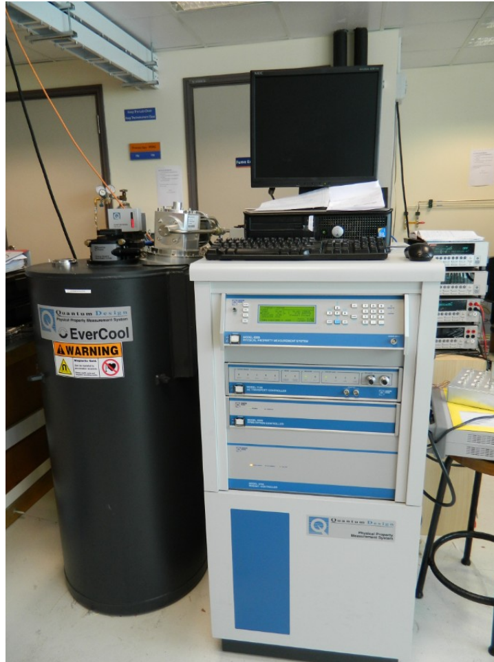
Figure 2.21. Photograph of the physical properties measurement system machine in our lab.
