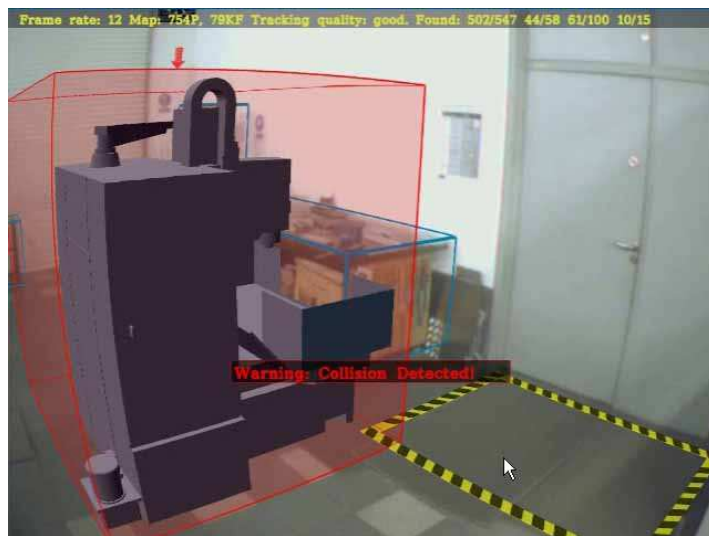
Figure 5.4.2: Simulated collision detection to assist manual planning
