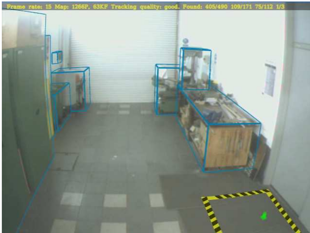
Figure 4.3.2: Models of existing facilities in a shopfloor
