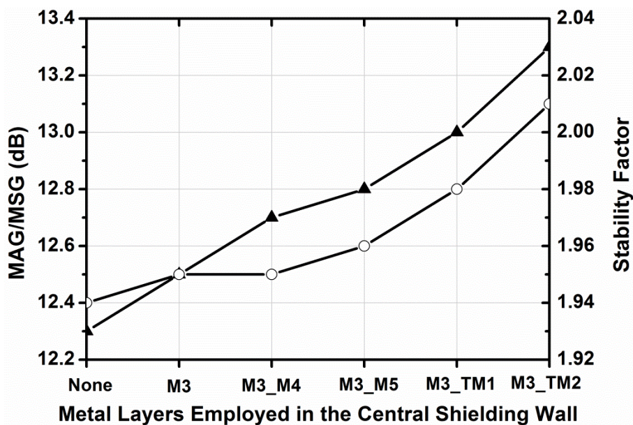
Figure 4.10: MAG/MSG and stability factor versus the height of the central shielding structure.
