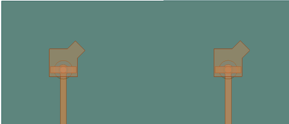
Figure 3-15 Array configuration of two adjacent stubbed patch antennas
