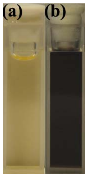
Figure 2.2 Digital photo of the supernatant derived from hydrothermal treatment of glucose in the presence of \text{KH}_2\text{PO}_4 (a) and in the absence of \text{KH}_2\text{PO}_4 (b).
