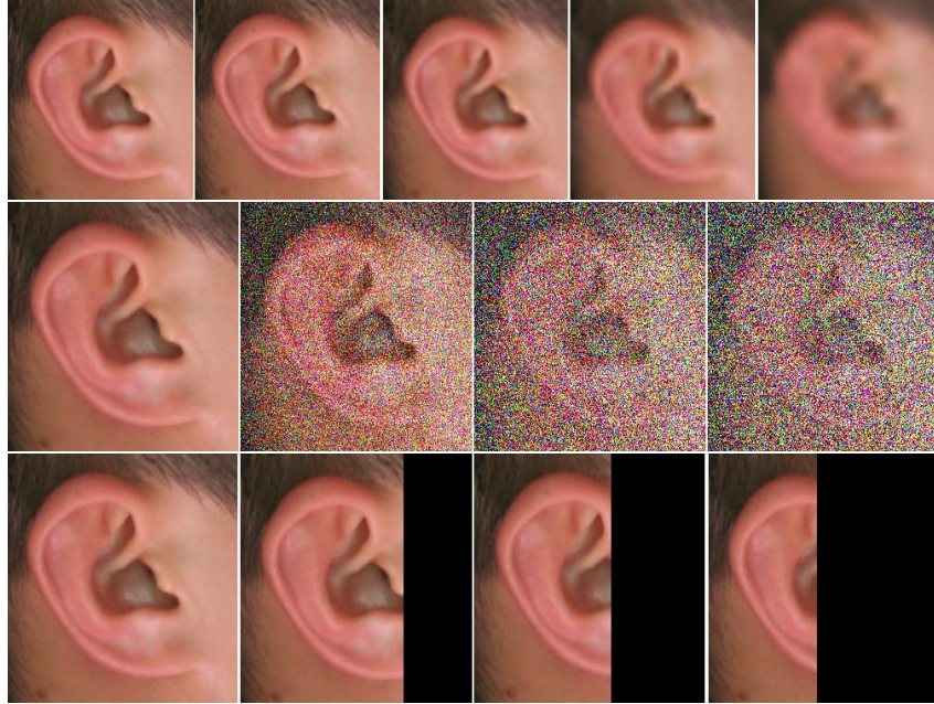
Figure 5.14: An example of resolution (left to right: 300 \times 300 , 150 \times 150 , 75 \times 75 , 37 \times 37 , and 18 \times 18 pixels), noise (left to right: standard deviation 0.0, 0.1, 0.3, and 0.5), and occlusion (left to right: 0%, 10%, 30%, and 50%) of ear images.
