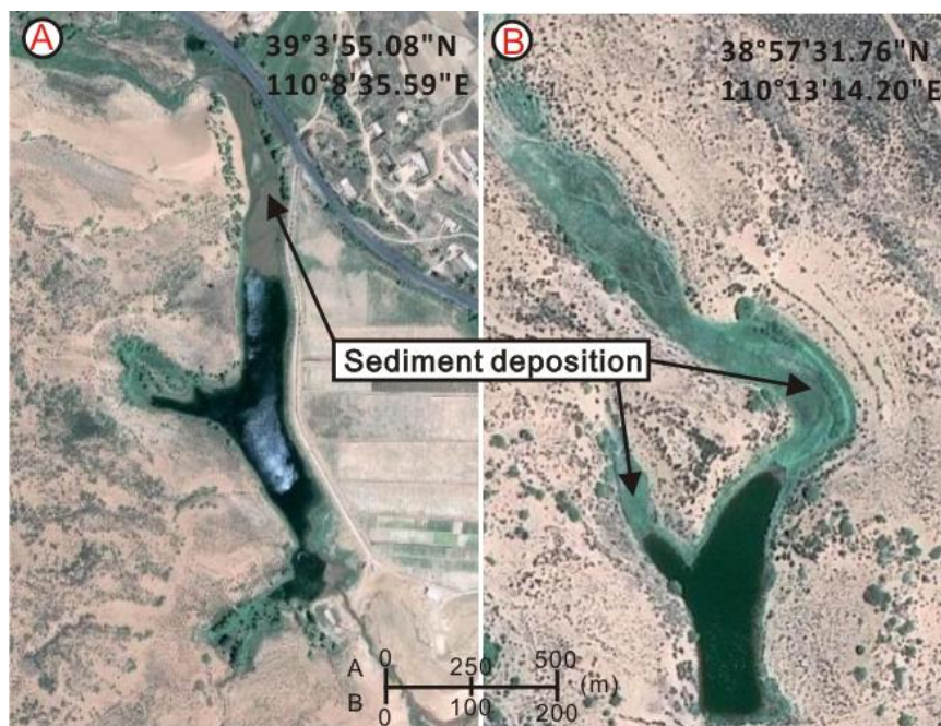
Figure 5.6 Two examples showing disappearing reservoir surface area due to sediment deposition.
