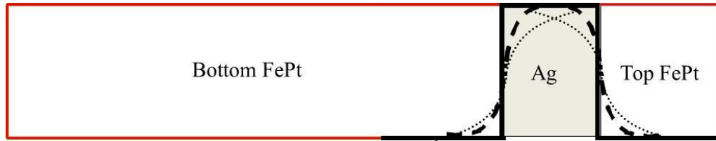
Figure 4.14 Schematic illustration of the dependence of Ag/FePt intermixing on intermixing factor a . Absence of intermixing when a = 0 (solid line). The extent of intermixing increases with increasing value of a , when a > 0 (dashed line to dotted line).
