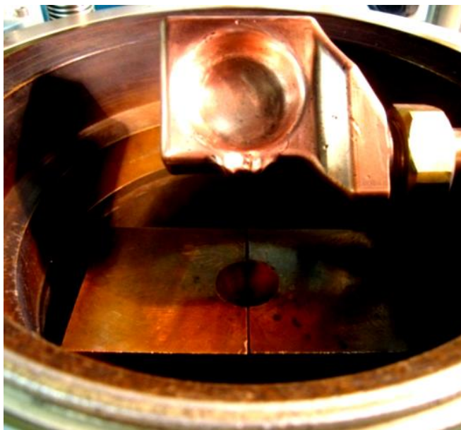
Figure 2.1 Optical image of the arc-melting furnace with a cylindrical copper mold of 5 mm in diameter.
